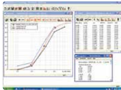
Quality control during measurement Comparison of the measurement result with upper and lower specification limits
