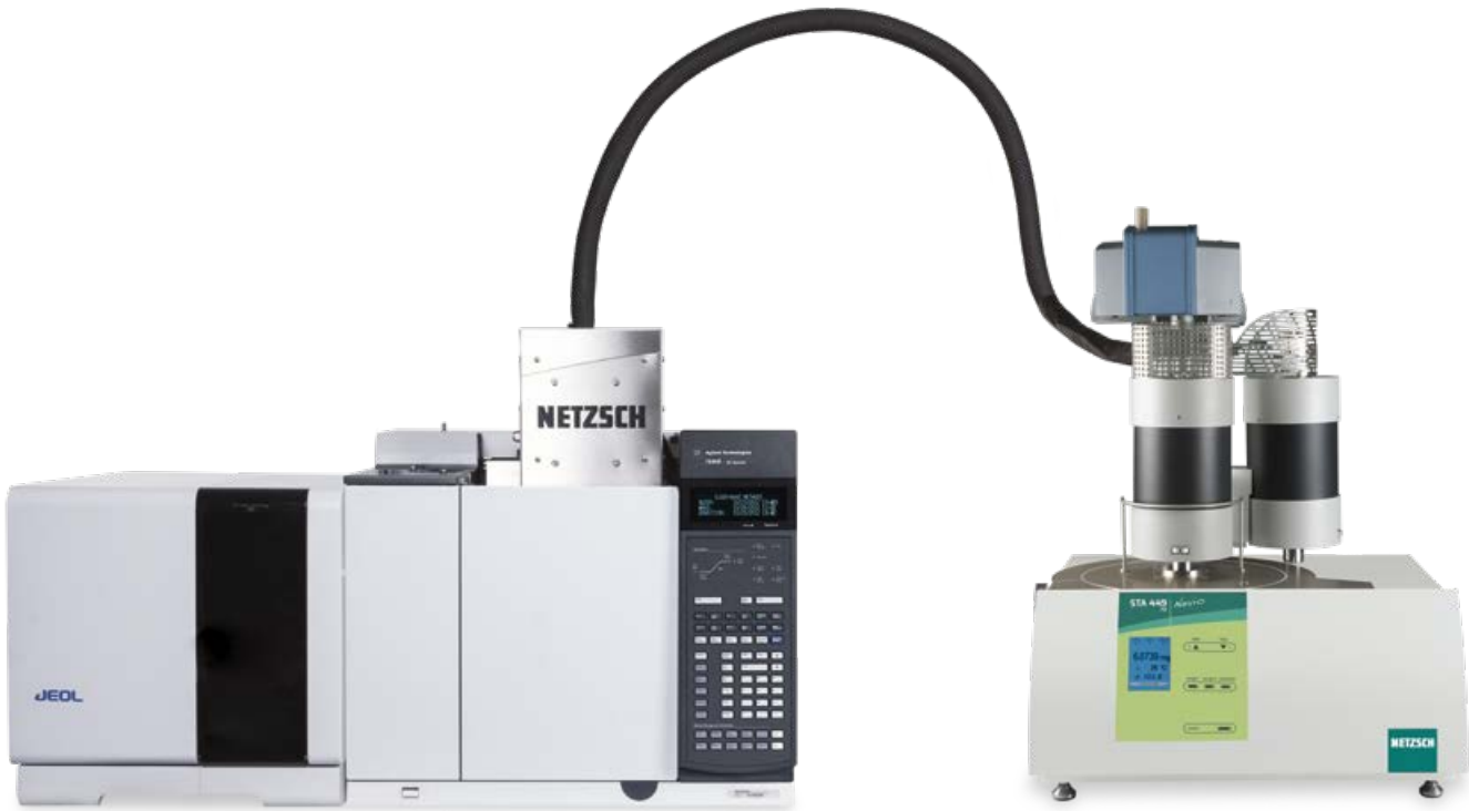
PERSEUS STA 449 F3 Nevio coupled to a GC-MS via capillary
