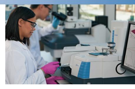
The Thermo Scientific Nicolet iS50R spectrometer carries forward all the flexibility and performance of the Nicolet™ iS™50 spectrometer system, with the added capabilities for the research spectroscopist. The Nicolet iS50R includes dual sources and triple detector optics, multiple on-board digitizers and easy access to spectrometer data and control signals.
