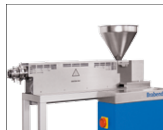
Measuring extruder 30/25 Application: Thermoplastics
