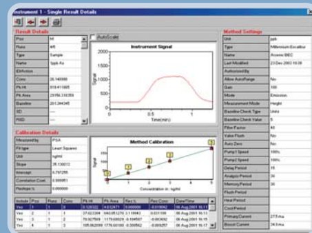
Ability to look at peak shapes during and after run. Peak shown 1ppb As
