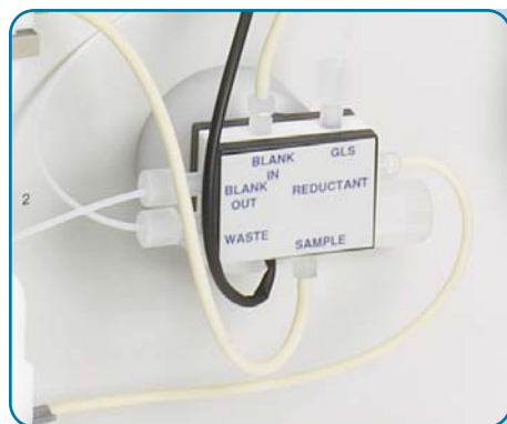
New valve concept to conserve reagents
